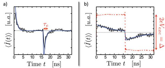
**Figure 4** Measurements of the average current in the time domain. The black traces represent the experimental points while the blue trace is an exponential fit. The escape times and average transmitted charges are  $\tau_e = 0.9$  ns,  $\langle Q_t \rangle = e$ , left panel,  $\tau_e = 10$  ns,  $\langle Q_t \rangle = 0.7e$ , right panel. The red dotted line represents the square excitation voltage.
