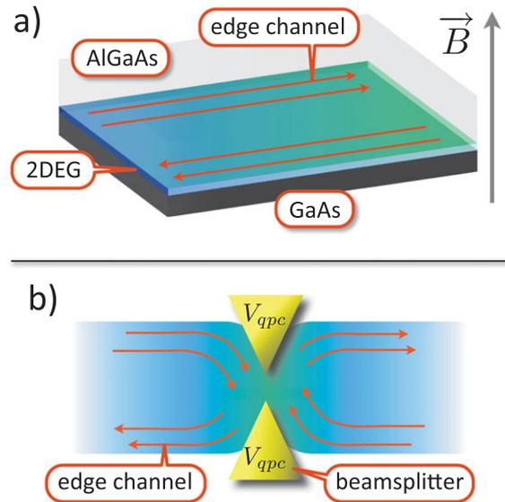
**Figure 1** a) Schematics of a 2DEG in the integer quantum Hall regime: when a strong perpendicular magnetic field is applied, electronic transport is governed by chiral edge channels. b) Schematics of a quantum point contact (QPC): when a negative voltage  $V_{qpc}$  is applied on split gates deposited above the 2DEG, a tunnel barrier is created and enables to realize the electronic analog of a beamsplitter.
